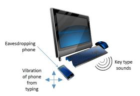
Fig. 3. Smart phone used as an eavsedropping device for nearby computing activity.
